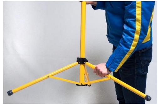
4.6.3 Loosen the screw on top of the tripod.
